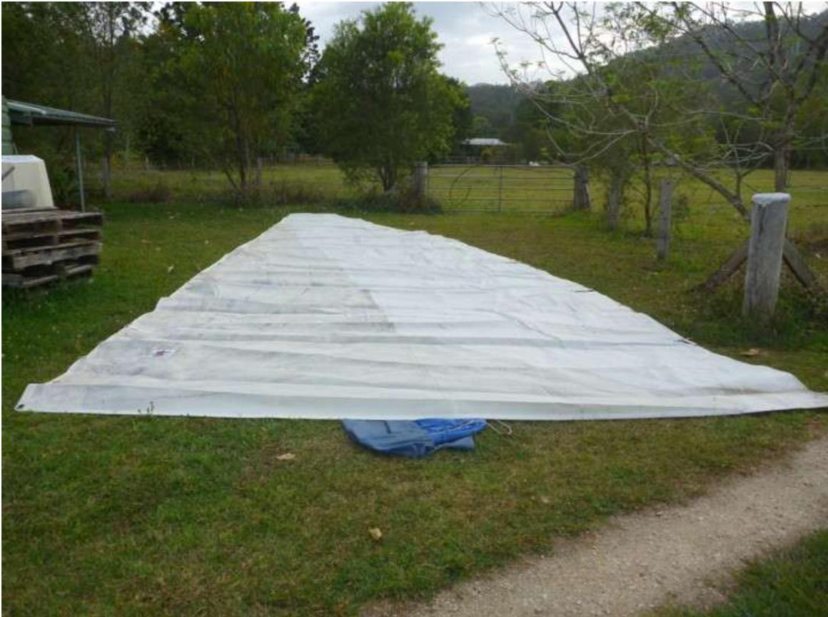
You can't see much from this pic but this is a pretty roachy main and is set up to be used with the Ronstan batten cars on the mast.
