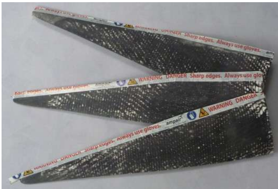
Ampair 300 blades Length – 550mm Weight – 314 grams each
