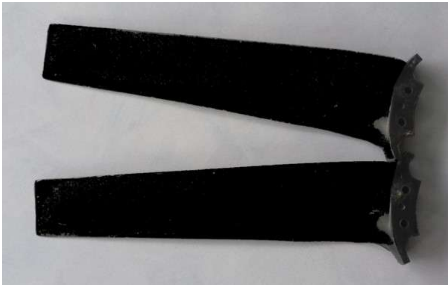
Ampair 100 blades Length – 380mm Weight about 195 grams each.
