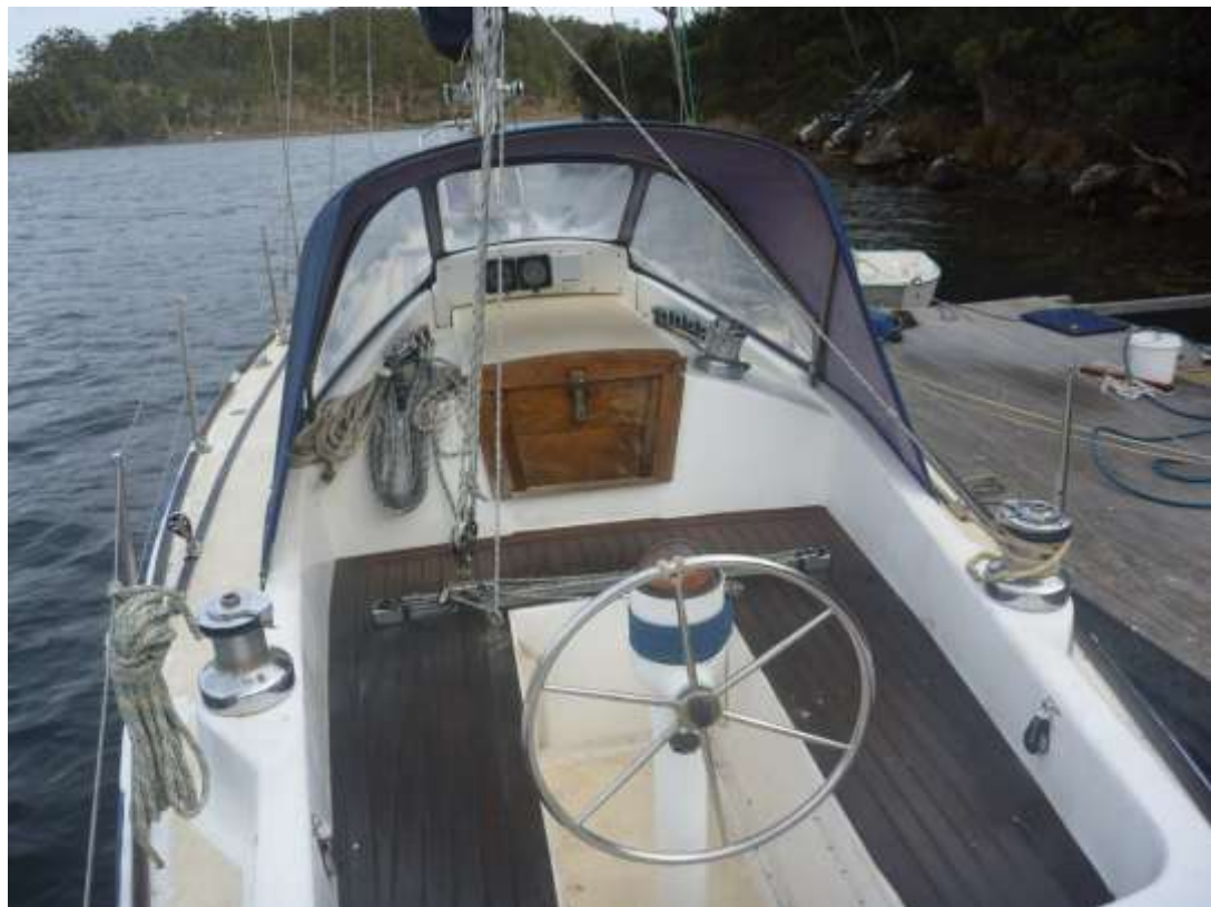
Note the smallish, uncluttered, cockpit, high storm step and small storm board. This boat was made to go to sea
